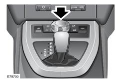
A rotary control just in front of the gear lever is used to select the required special program. When the selector reaches the end of the selection range in either direction it can be rotated further, but it has no effect.
