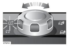
When the starter button is pressed, the indicators around the rotary control are illuminated. The active program is highlighted in amber, and the program icon is displayed in the message centre.
